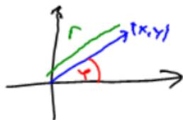
$$g'(r, \varphi) = \begin{pmatrix} \cos \varphi & -r \sin \varphi \\ \sin \varphi & r \cos \varphi \end{pmatrix} \quad \det g'(r, \varphi) = r$$
